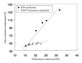
Properties 5. Dependence of  $T_g$  on norbornene content of E/N and E/N/3<sup>rd</sup> monomer copolymers initiated with  $iPr(Cp)(Flu)ZrCl_2$  and MMAO-4 catalyst system.
