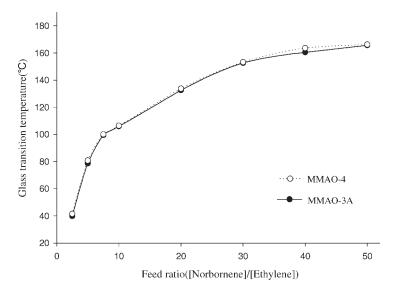
**Figure 3.** Effect of MMAO cocatalyst types on  $T_g$  of E/N copolymer obtained with  $iPr(Cp)(Flu)ZrCl_2$  ([Zr]=2.5 × 10<sup>-5</sup>mol/L, [Al]/[Zr]=3000, 40 °C, 1atm, 1h).
