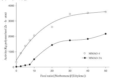
Figure 2. Effect of MMAO cocatalyst types on catalytic activity for E/N copolymerization initiated with  $iPr(Cp)(Flu)ZrCl_2$  ( $[Zr]=2.5 \times 10^{-5}mol/L$ , [Al]/[Zr]=3000,  $40^{\circ}C$ , 1atm, 1h)
