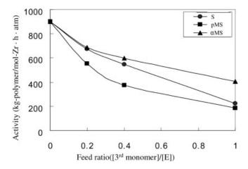
Figure 4. Effect of 3<sup>rd</sup> monomer addition on catalytic activity initiated with  $iPr(Cp)(Flu)ZrCl_2$  and MMAO-4 catalyst system. (Polymerization conditions:  $[Zr]=2.5\times10^{-5}$  mol/L, [Al]/[Zr]=3000, [N]/[E]=2.5, 40 °C, 1 atm, 1h)
