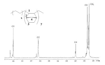
**Figure 1.**13C-NMR spectrum of E/N copolymer obtained with iPr(Cp)(Flu)ZrCl<sub>2</sub> and MMAO-4 cocatalyst ([N]/[E] feed ratio = 10/1)
